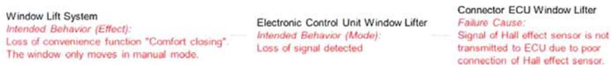
Figure 4.4-6 Example of a structure with hybrid failure chain including a monitoring which always is effective and switches the system to a mitigated Failure Effect (scenario (3))
