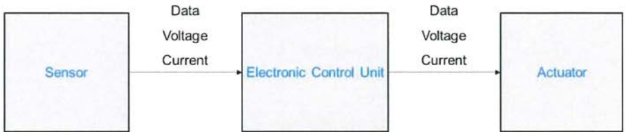
Figure 4.1-1 Generic block diagram of an Electrical / Electronic / Programmable Electronic System
