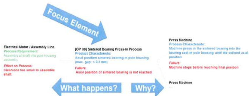
Figure 3.4-2 Example of Failure Analysis Structure Tree
