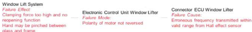
Figure 4.4-5 Example of a structure with failure chain without a monitoring or with a monitoring which is only partially effective (scenario (1) and (2)).
