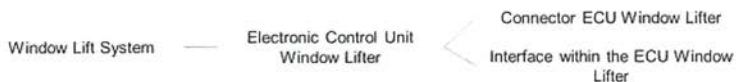
Figure 4.2-1 Example of a structure tree of a window lift system for investigating erroneous signals, monitoring, and system response
